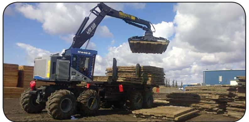
TimberPro 840 with a custom grapple. Loading and transporting rig mats.
